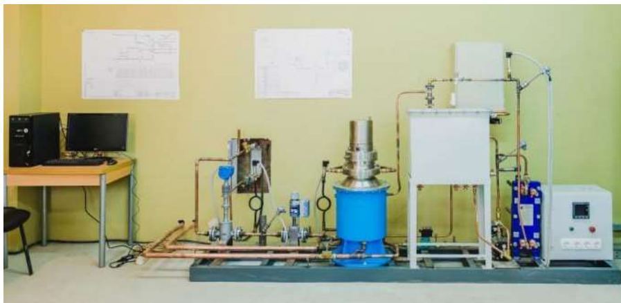
Microturbine complex developed by department staff
